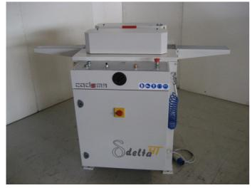
Vertical polishing machine Max. workable thickness 60 mm
