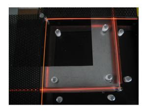
Small table top heating machine to obtain boxes, both square and rectangle, with min dimensions 90 x 90mm and max 450 x 450mm.
